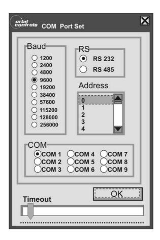
The Timeout sliders have to be set in accordance with the speed of the PC. The setting shown above fulfils the most applications. The settings must be terminated with OK!
